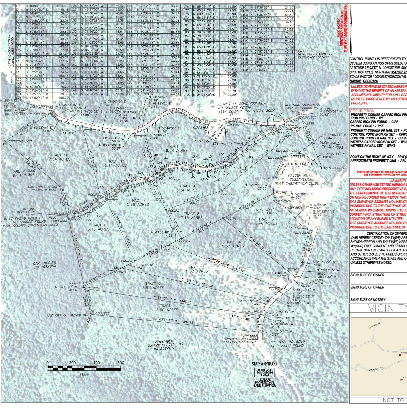
CONTROL POINT 1 IS REFERENCED TO THE NATIONAL SPATIAL REFERNCE SYSTEM USING AN NGS OPUS SOLUTION OF <u>08/12/2015@12:31 PM</u> SPC (1600 KY1Z) NORTHING <u>3547007.27'</u> EASTING <u>5286034.76'</u> SCALE FACTOR1.00000627HORIZONTAL DATUM NAD83 VERTICAL DATUM
